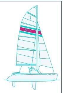
Construction: Fiberglass/Foam Core sandwich composite. Vacuum bag lamination. Aluminum spars and stainless steel wire rigging.
